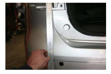
Position cardboard template on this mark. Making sure template is on the correct way. (TOP) is up and (L) or left is facing toward centre of vehicle. Wrap template around bumper corner following natural line in bumper. At the mark, flip the template over and mark right hand side the same way.
