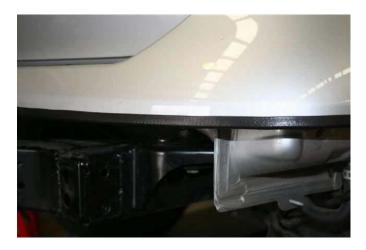
15. On either side of chassis, are two captive nuts, knock out nuts, then drill holes to  $\frac{1}{2}$ ".
