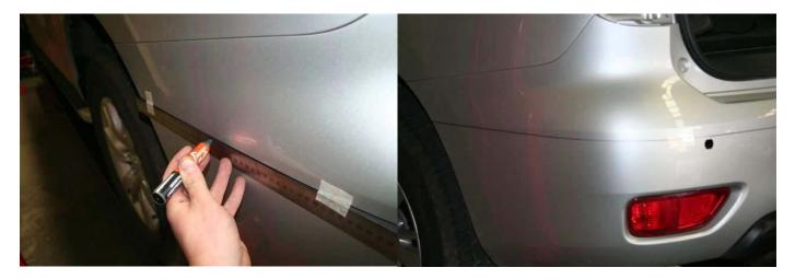
13. Check all measurements are correct. Then using a grinder with cutting disc. Cut on line. If cutting bumper while bumper is on vehicle, be careful not to cut through any vehicle wiring eg:- sensor harness.
