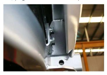
18. Fit 4 x 2 either side – bolt on wire, through rectangular hole in chassis out through holes you drilled earlier using M12 flat, spring and nut.
