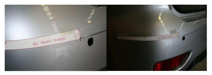
12. Measure down from where bumper meets body at wheel arch 100mm. Mark and with a ruler join line across to where template line finished.
